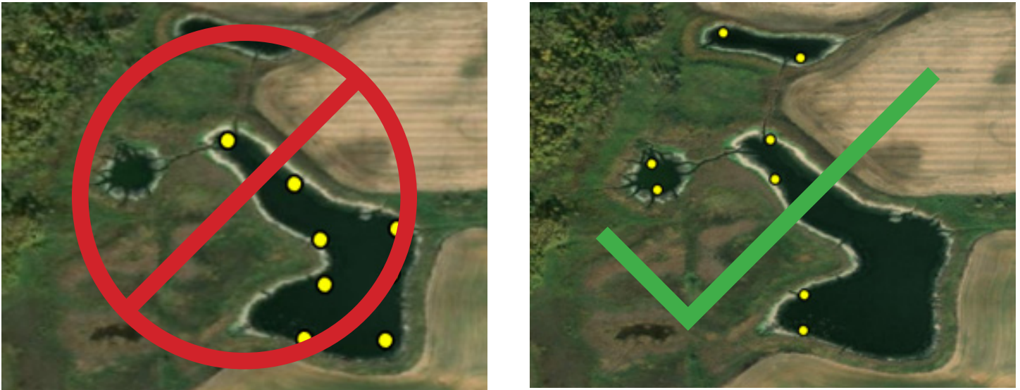
Figure 4. The Hen House deployment in the photo to the right will have a higher usage and the structures will be less likely to suffer ice damage.
